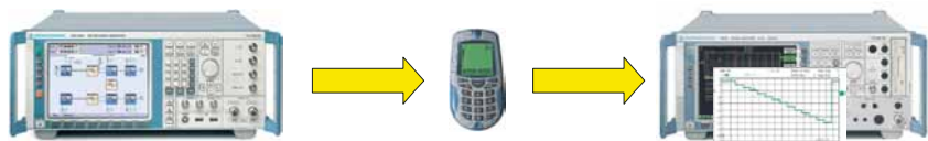
The mobile phone changes its output power in compliance with TPC information from the R&S SMU200A
